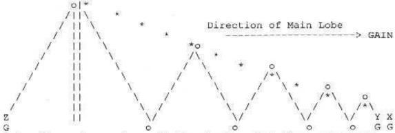
Note: Space does not permit the display, but there are seven points "o" at ground level and eight above ground. In other words, there are eight "triangles" in the featured antenna while only five are shown above.
