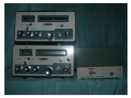
Requires an 8-conductor cable, 8-pin plug, 11-pin socket (to connect HX-20 to the HR-20).
