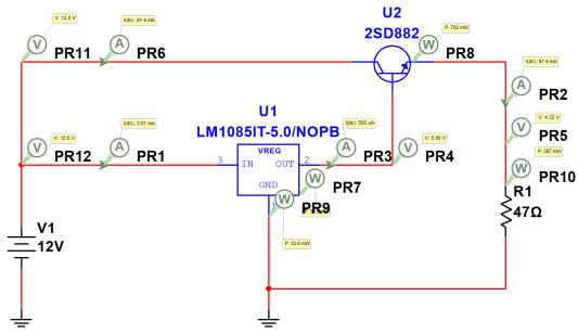
The schematics is simple, but one of the problems is I do not obtain 5 Volt at the output, but 4.32 Volt, and no longer so stabilized as the 5V IC could do it. The solution is to arrange a different schematic, with a pnp transistor. The drawing and simulation are also done by me in Multisim 14.3:
