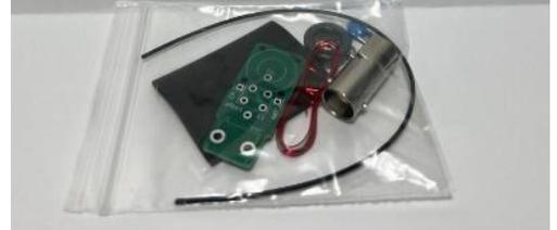
To say this is a tiny QRP antenna transformer understates the truth. This kit takes QRP to the next level of small and lite. Options on the commercial kit include build it as a 9:1 or 49:1 depending on your preference.
