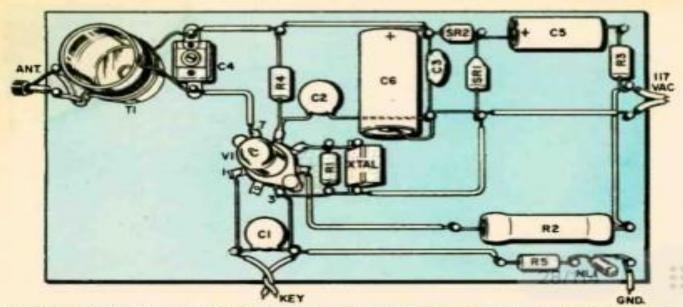
Our model, built on 6 x 10 x %-in,-thick piece of pine, has 23 finishing-nail tie points. V1's socket alts on %-in, spacers; carpet tacks hold it in place. Contacts from discarded tube socket hold crystal.
